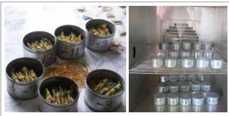
Figure 5. Plant parts placed in sand-filled containers for cold tests and placed in the freezer (Original).
